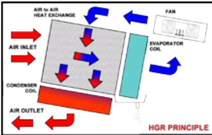
Humid air is drawn into the dehumidifier and passes through an "Air to Air" Heat Exchange.
